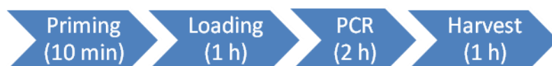
Figure 26. Workflow. Priming and loading of the 48.48 Access Array™ takes place in a Pre-PCR IFC Controller AX. The Access Array is transferred to FC1 Cycler for PCR, and PCR-products are harvested in a Post-PCR IFC Controller AX (Fluidigm).
