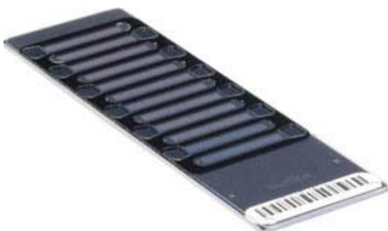
Figure 18 shows a BeadChip where 6 samples can be loaded with a multi-channel precision pipette into the left side of the BeadChips, and 6 samples into the right side according to a loading protocol. On the top of the BeadChip a unique Barcode is placed.
