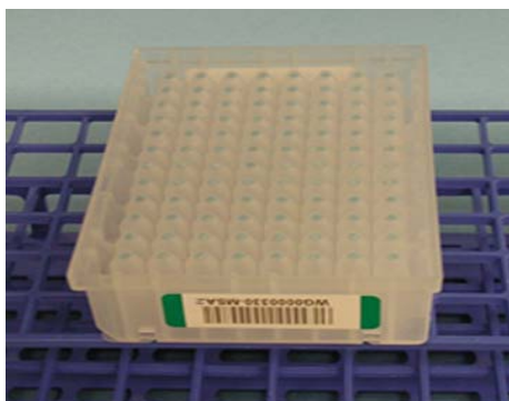
Figure 16 An uncovered MSA2 Plate Inverted for Air Drying. The blue pellets are shown in the bottom of the wells
