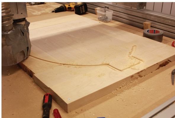
Here the cutter was positioned in the middle of the object and a height was set to start machining.
