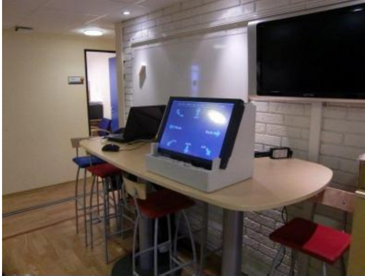
Fig. 4. The self-service kiosk prototype implemented using a touch display mounted in a polystyrene case.
