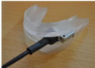
Figure 8. Fixation of the optical probe by means of a gum shield.
